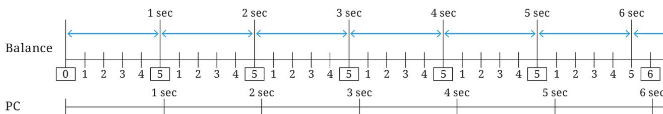
**Time disparity of two different internal clocks** (when the balance display refresh rate is 5 times/sec, the calculation time is 1 sec, and the balance's internal clock goes slightly ahead of the PC's)
