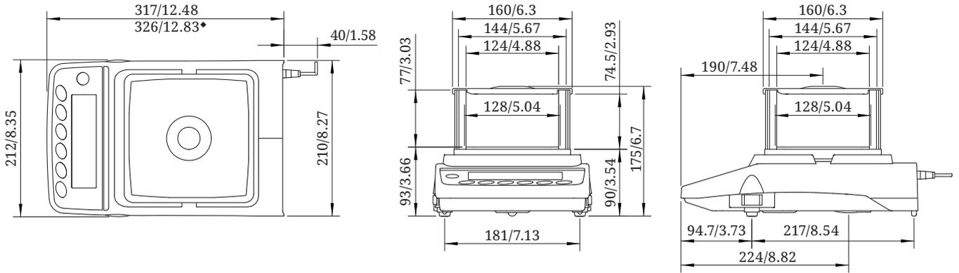
**0.01/0.1 g models** | GX-2002A / GX-3002A / GX-4002A / GX-6002A / GX-10002A / GX-6001A / GX-10001A
