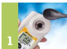
1 Place the sample onto the prism surface.
